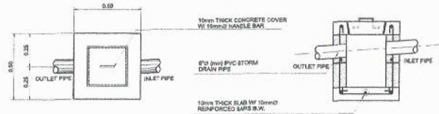
2 CATCH BASIN/JUNCTION BOX DETAIL SCALE: 1/4" = 1'-0"
