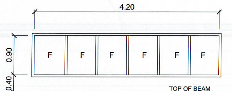
W 9 ALUMINUM FIXED WINDOW COMPLETE W / ALL ACCESSORIES W / 3/8" THK. TEMPERED GLASS 6 SETS
