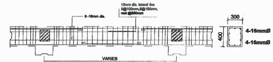
DET. OF FOOTING TIE BEAM 1 SCALE NTS.
