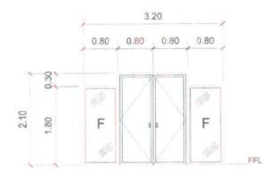
1 - 1,50M X 2.10M DOUBLE SWING DOOR WITH 2 - 0.80M X 1.80M FIXED GLASS, TEMPERED GLASS ON A 50MM POWDER - COATED ALUMINUM FRAME, FEATURING ONE WAY GLASS AND COMPLETE ACCESSORIES. 2 SETS (ENTRANCE AND EXIT)
