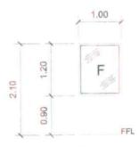
1.00M X 1.20M FIXED GLASS ON A 50MM POWDER - COATED ALUMINUM FRAME, TEMPERED GLASS, FEATURING ONE WAY GLASS AND COMPLETE ACCESSORIES. 1 SET (CONFERENCE ROOM)
