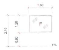
1.60M X 1.20M FIXED GLASS ON A 50MM POWDER - COATED ALUMINUM FRAME, TEMPERED GLASS, FEATURING ONE WAY GLASS AND COMPLETE ACCESSORIES. 1 SET (CONFERENCE ROOM)
